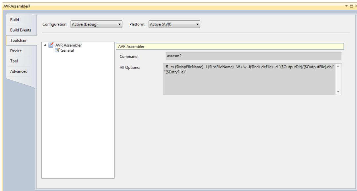
Figure 3-27. Assembler Setup Dialog, General Options Shown
