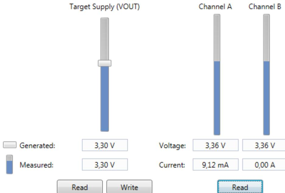
The voltage output (VOUT) is adjusted by the slider, or by typing a voltage in the **Generated** text boxes below the slider.
