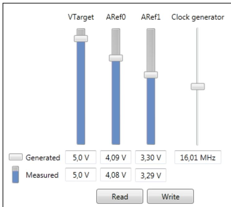
The set-points of the three voltage sources (VTG, ARef0, and ARef1) are adjusted by the means of three sliders. It is also possible to type a voltage in the **Generated** text boxes below the sliders. When you drag the sliders, the text boxes will update. And when you type a value in the text box, the slider will move.
