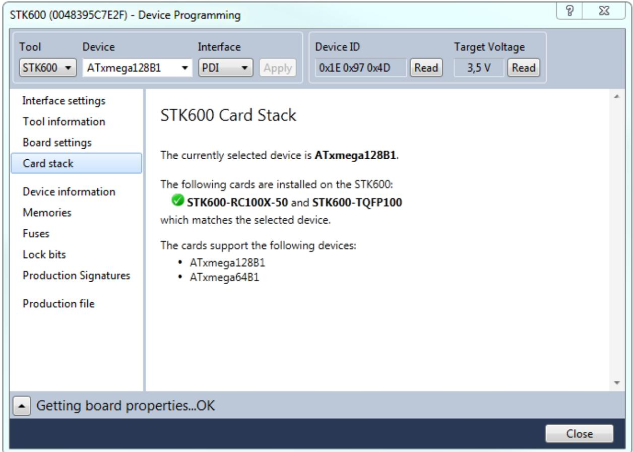
The card stack page tells which cards are mounted on the STK600 and if they support the selected device. If they do match, a list of devices supported by that card combination is listed.
